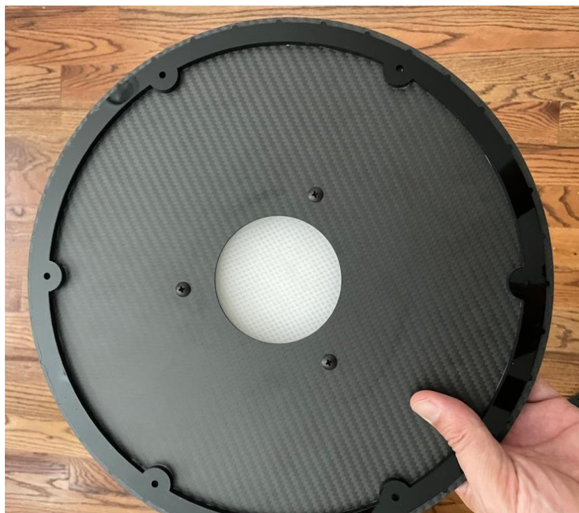
Figure 32: back plate of Moana, inside side, showing the coupling mechanism fitting the inside of the OTA.
