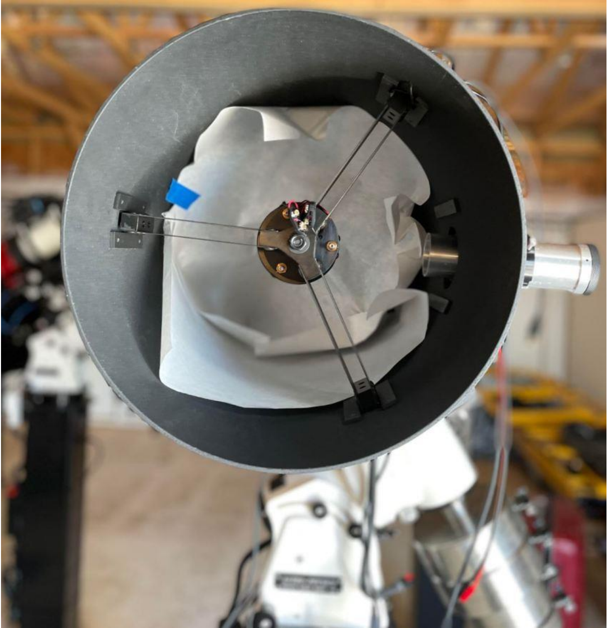
Figure 27: front view of the telescope during collimation (secondary centering).
