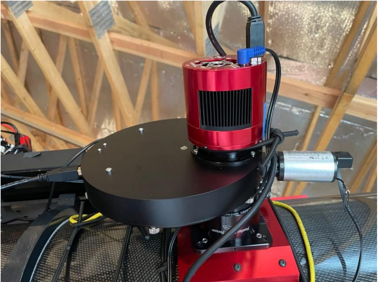
Figure 30: focuser, filter wheel, guide and imaging camera.
