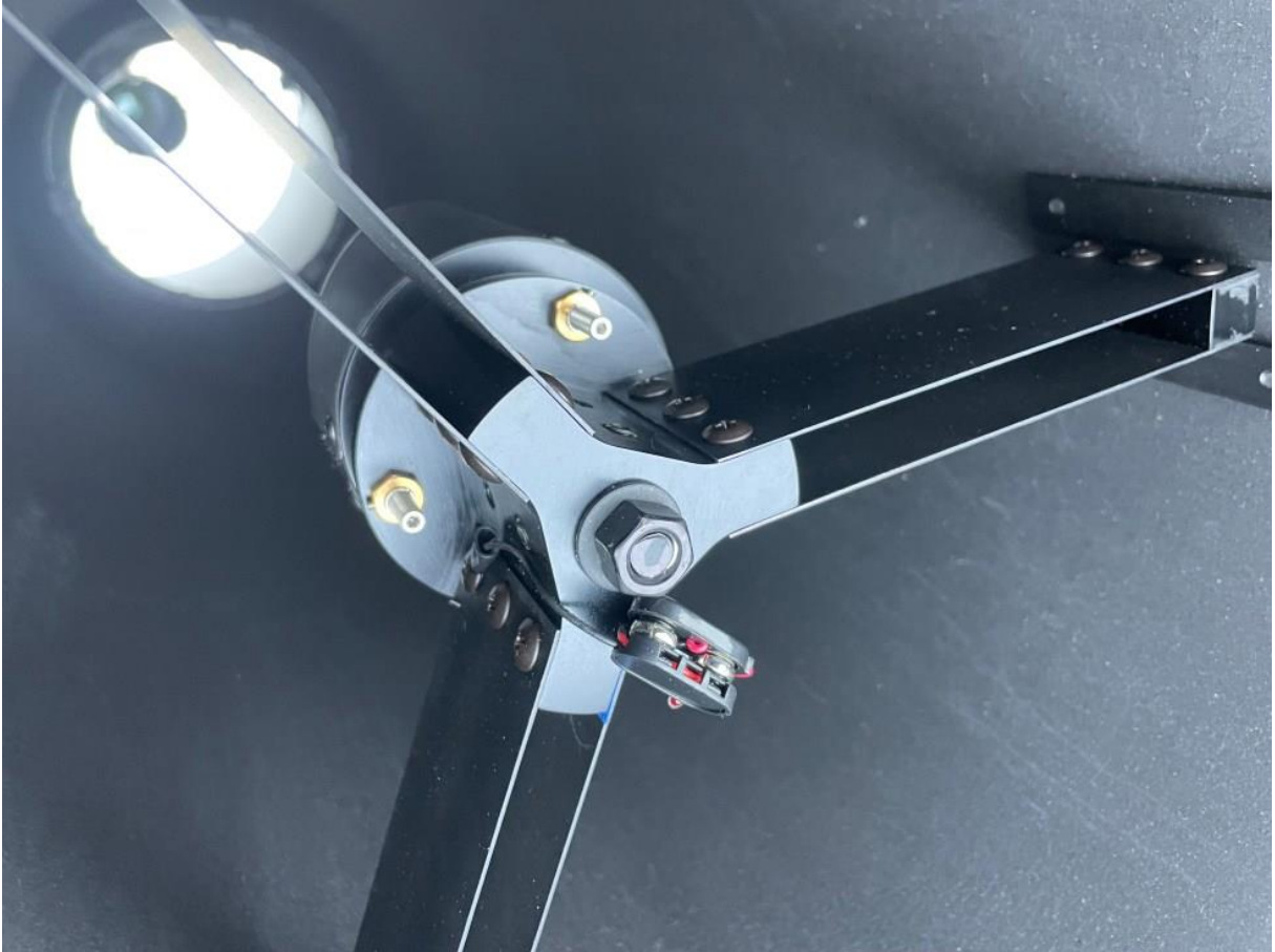
Figure 22: double van spider and secondary assembly.
